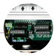
Plug-in terminal connection for easy wiring.
