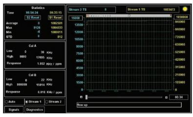
figure 2. A 33-minute run at 100% sulfur with a standard deviation of 812, indicating excellent repeatability.
